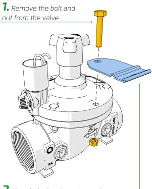
**2.** Attach the bracket adapter plate to the valve using the bolt and nut which were removed
