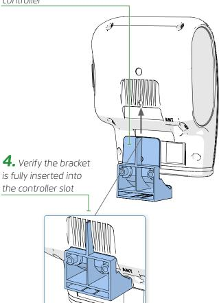
**5.** Position the mounting bracket onto the bracket adapter plate
