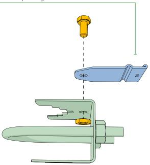
**2.** Attach the U-clamp to the pole using two nuts
