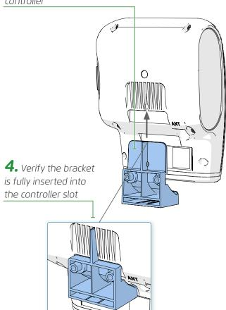
**5.** Position the mounting bracket onto the bracket adapter plate **6.** Verify the bracket adapter plate clicks in place and is securely fastened to
