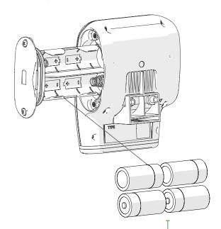
Insert four batteries according to the orientation shown in the battery compartment
